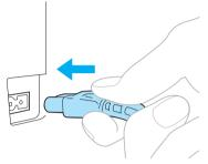
Insert the plug of the power supply cord into a household electrical outlet.
